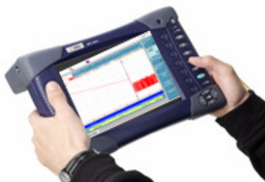
6. MTS/T-BERD 6000 platform with OTDR module
